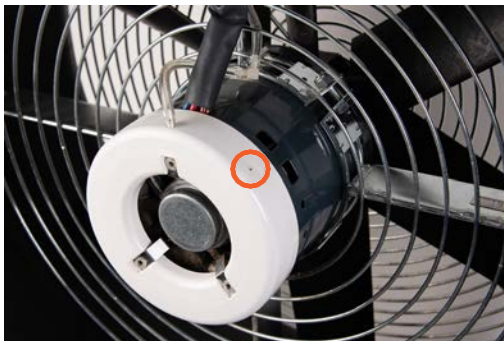
Figure 5. Pressure sensor used to measure airflow through the blower door fan.
