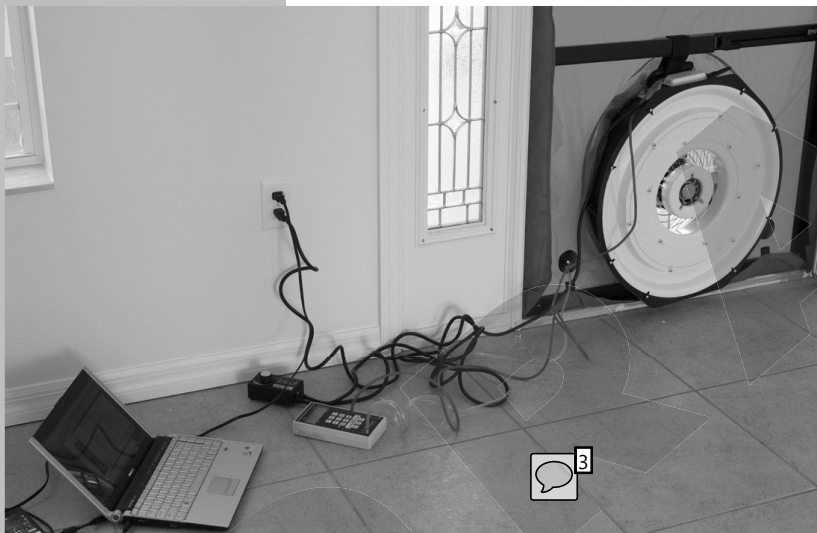
Blower door set up for an air leakage test.
