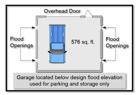
Let's look at an example. We have a garage of 576 square feet. Therefore, a total of 576 net square inches of relief opening is required. With four openings provided, each opening is required to provide a minimum of 144 square inches.
