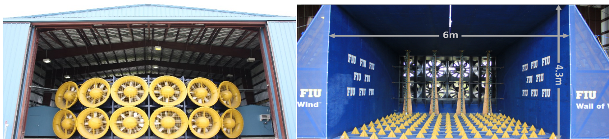
Figure 2. The 12-fan and floor roughness elements of the Wall of Wind (WOW) facility.
