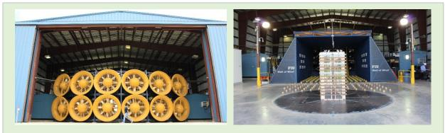
Figure 1 - NHERI 12-Fan Wall of Wind Experimental Facility: (a) Intake side, (b) Open jet test-section side.
