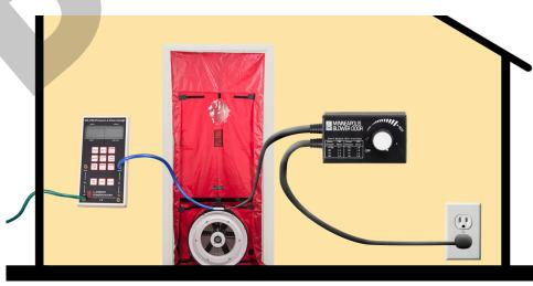
Figure 6. How blower door components are connected.
