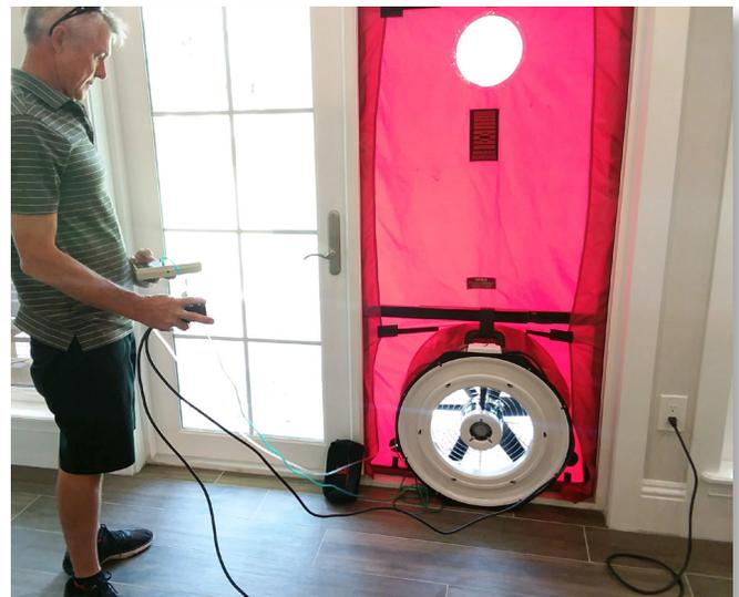
Test results are reported on a form that includes space to record the home's CFM50 measurement, conditioned volume, ACH50 value and Pass/Fail status, and an area for the tester to provide their name, company, qualification and signature. A blank Building Officials Association of Florida
