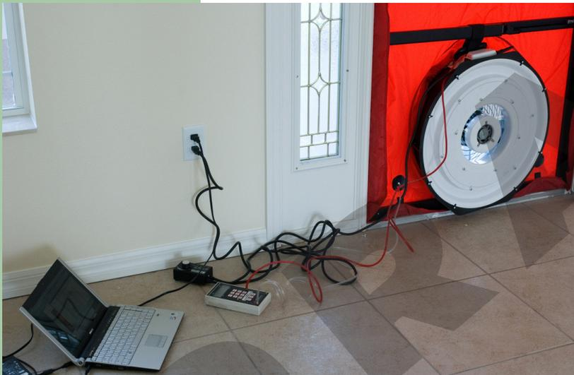
*Blower door set up for an air leakage test.*
