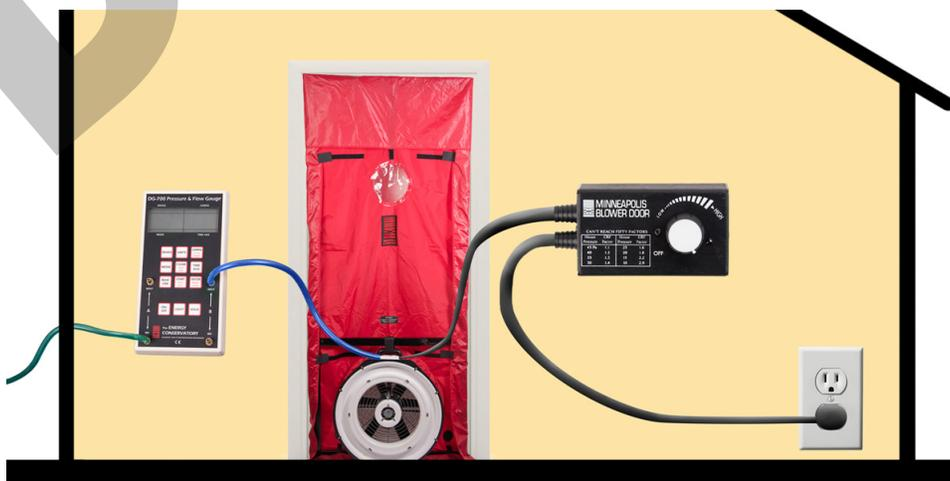
Figure 6. How blower door components are connected.
