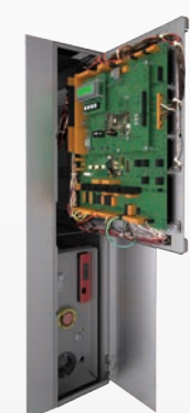
CONTROL PANEL IN DOOR JAMB
