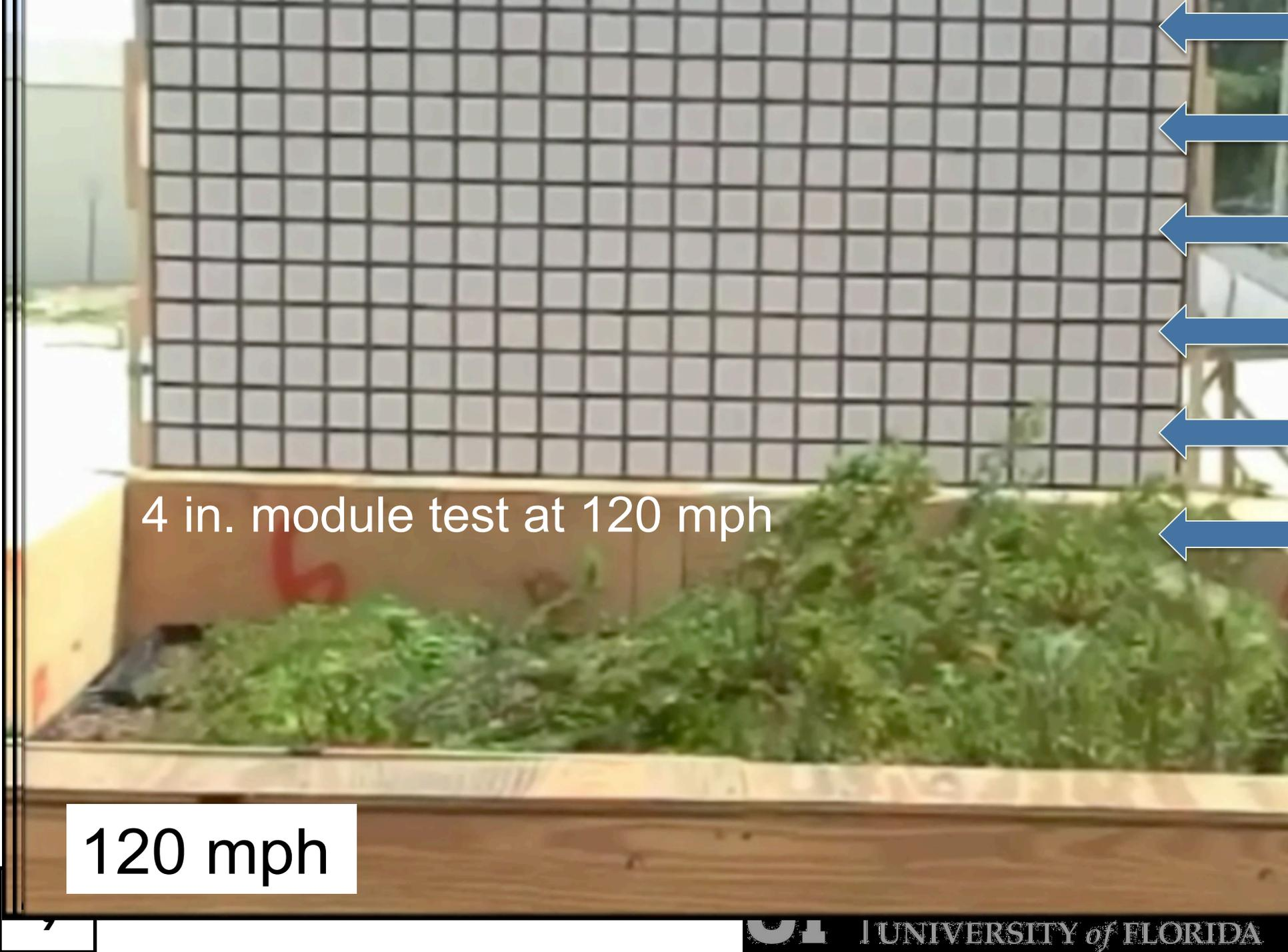
4 in. module test at 120 mph
