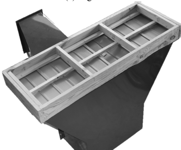
(b) Airbox for Testing of Straight Sections
