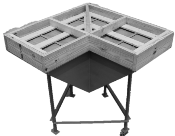
(c) Airbox for Testing Corner Sections (Service Port in Rear)
