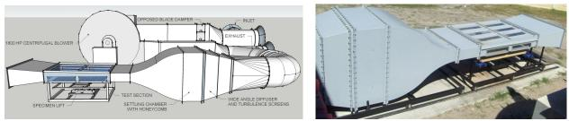
Figure 1. Dynamic Flow Simulator a) componentry and b) as constructed.
