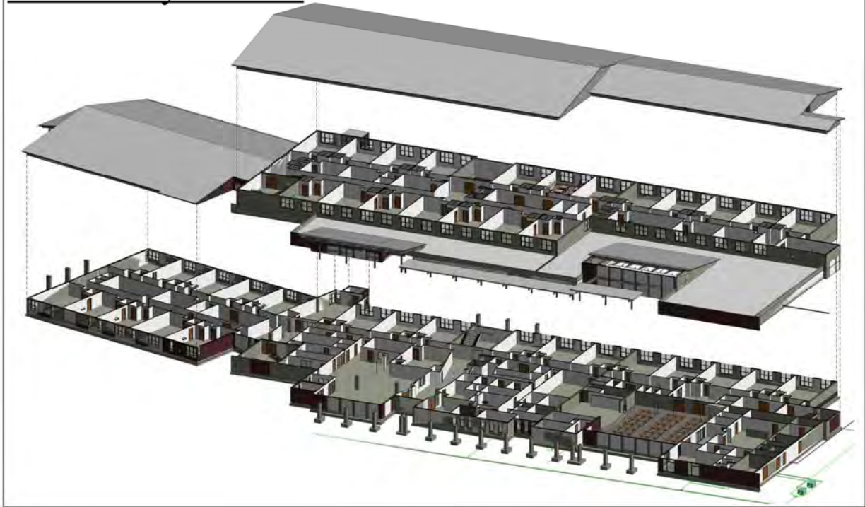
Figure C-1. 3D sections of Elementary School
