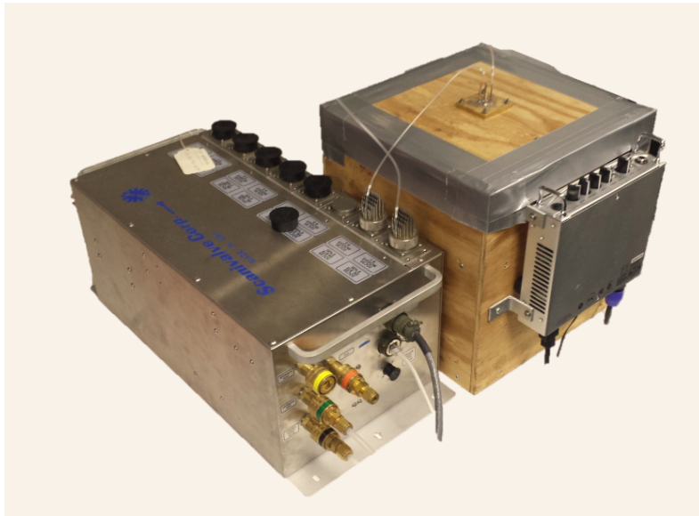
Figure 5. Tubing frequency response correction test setup. 512-channel pressure scanning system (left) and pneumatic frequency signal source box with amplifier (right).
