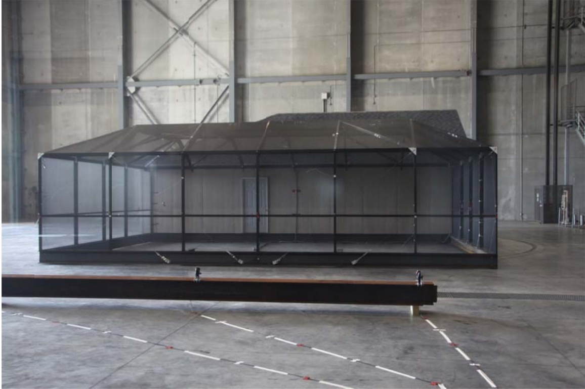
Figure 7. AAF specimen in the testing chamber
