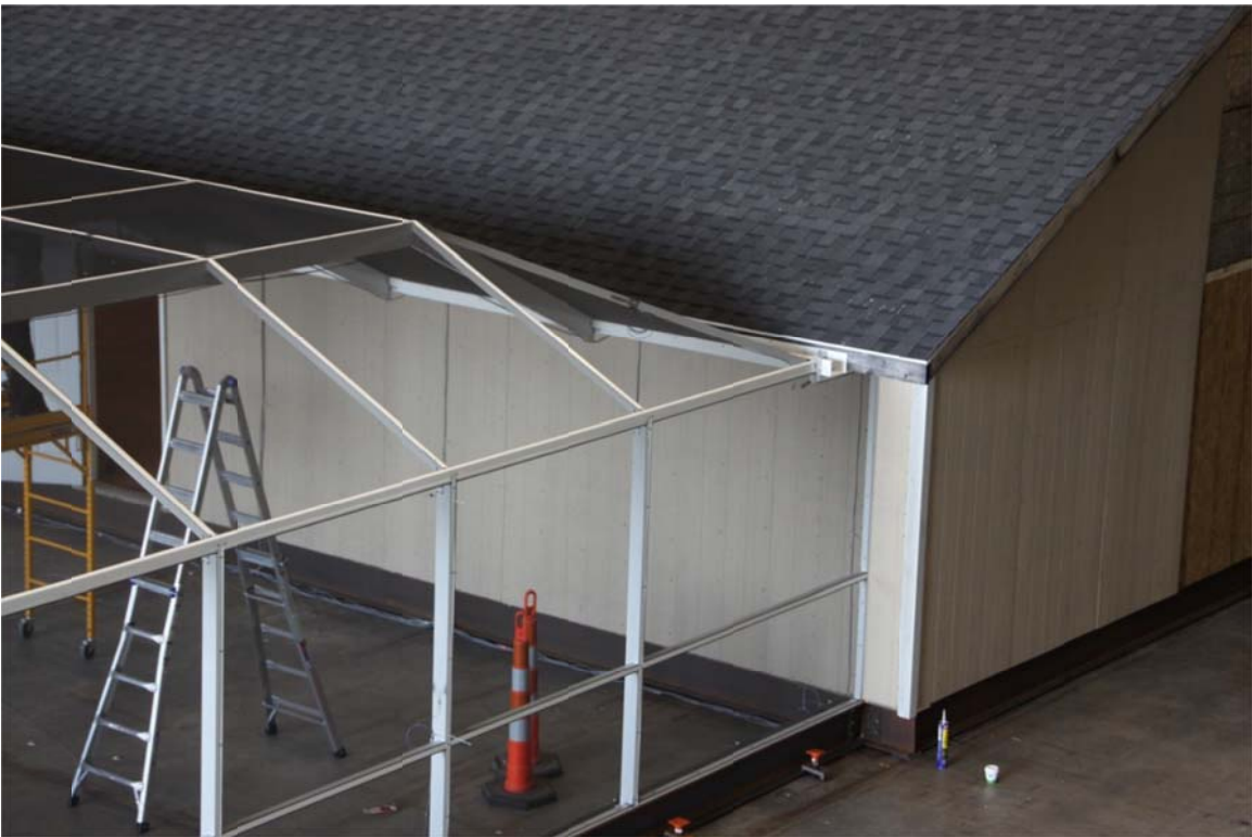
Figure 6. Specimen attachment to the host structure and the foundation
