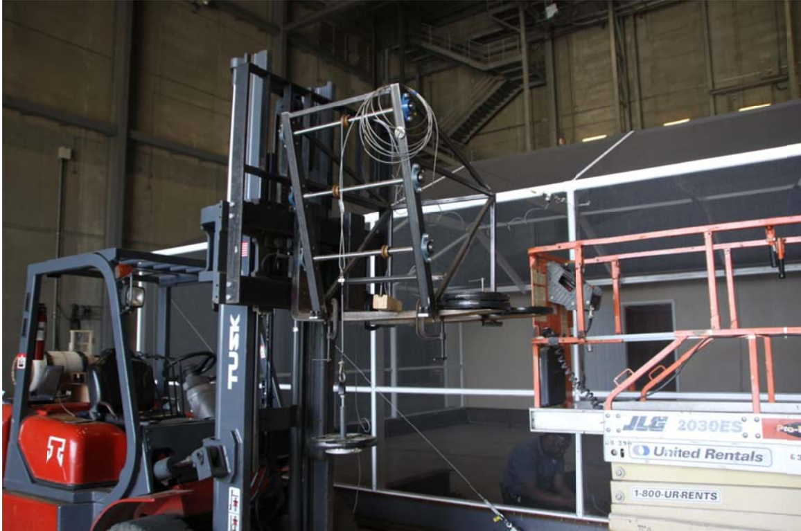
Figure 14. The apparatus for applying the static point load
