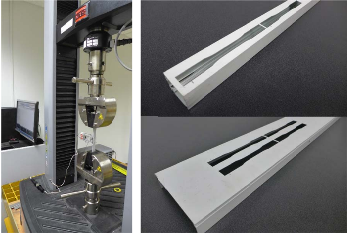
Figure 29. Material testing machine (left) and 2X2 and 2X6 SMB after harvesting testing coupons (right)
