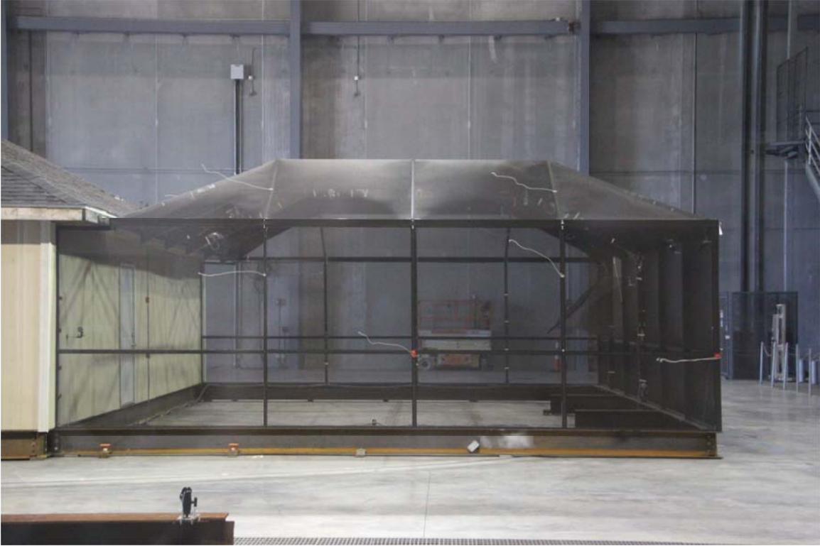
Figure 23. Failure of the screen attachment during Run 29 (maximum wind speed = 90 mph)
