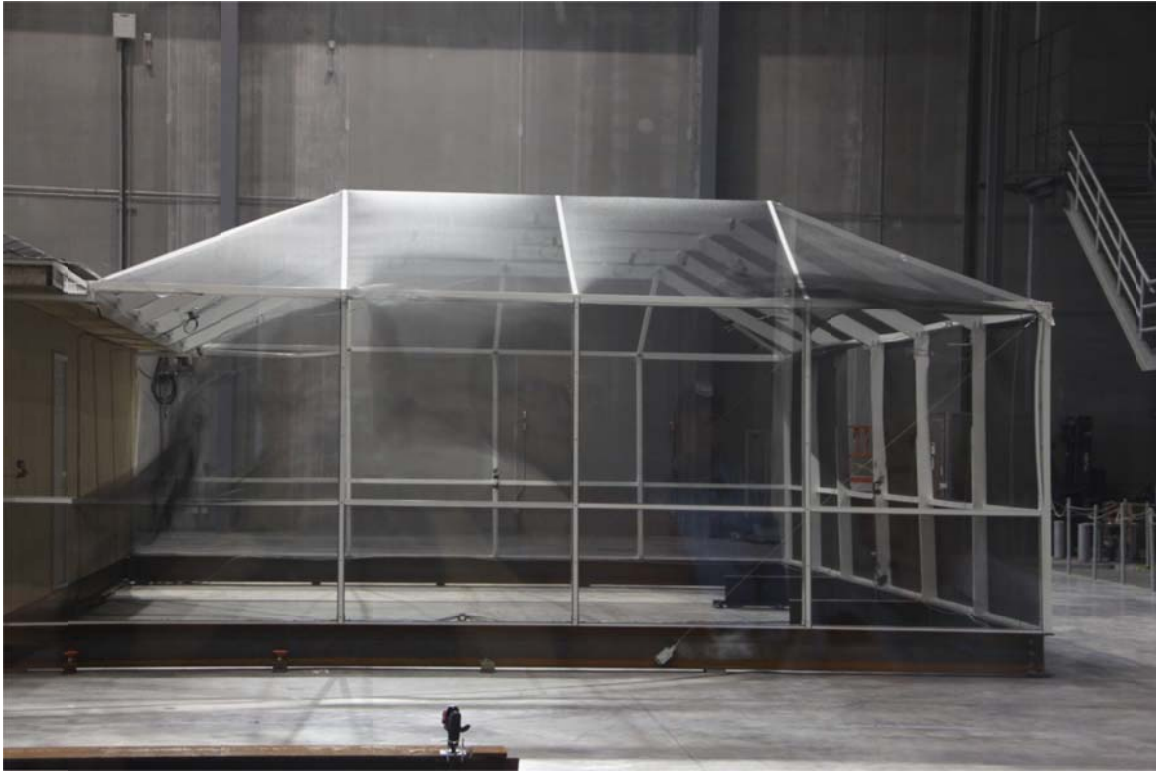
Figure 21. Failure of the screen attachment during Run 32 (maximum wind speed = 100 mph)
