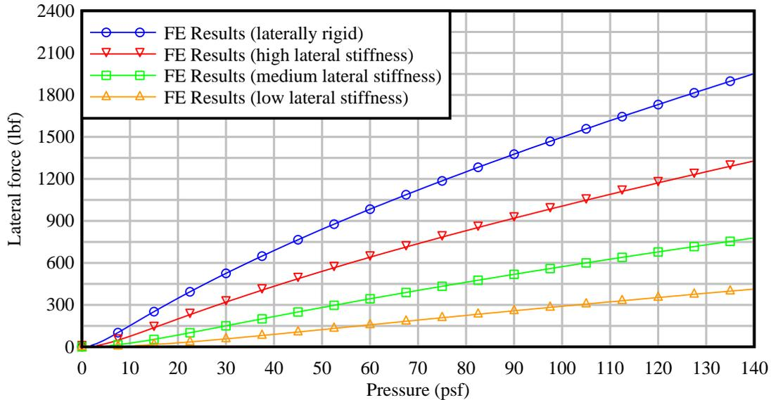
Figure 5. Comparison between FE lateral force results for different lateral stiffnesses in the toward-the-building load direction
