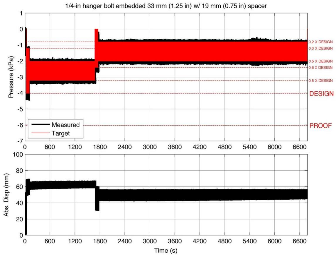
Figure 18. Cyclic pressure loading sequence derived from ASTM E1996 for Case 2 (1.25 inch embedment) for the negative pressure case
