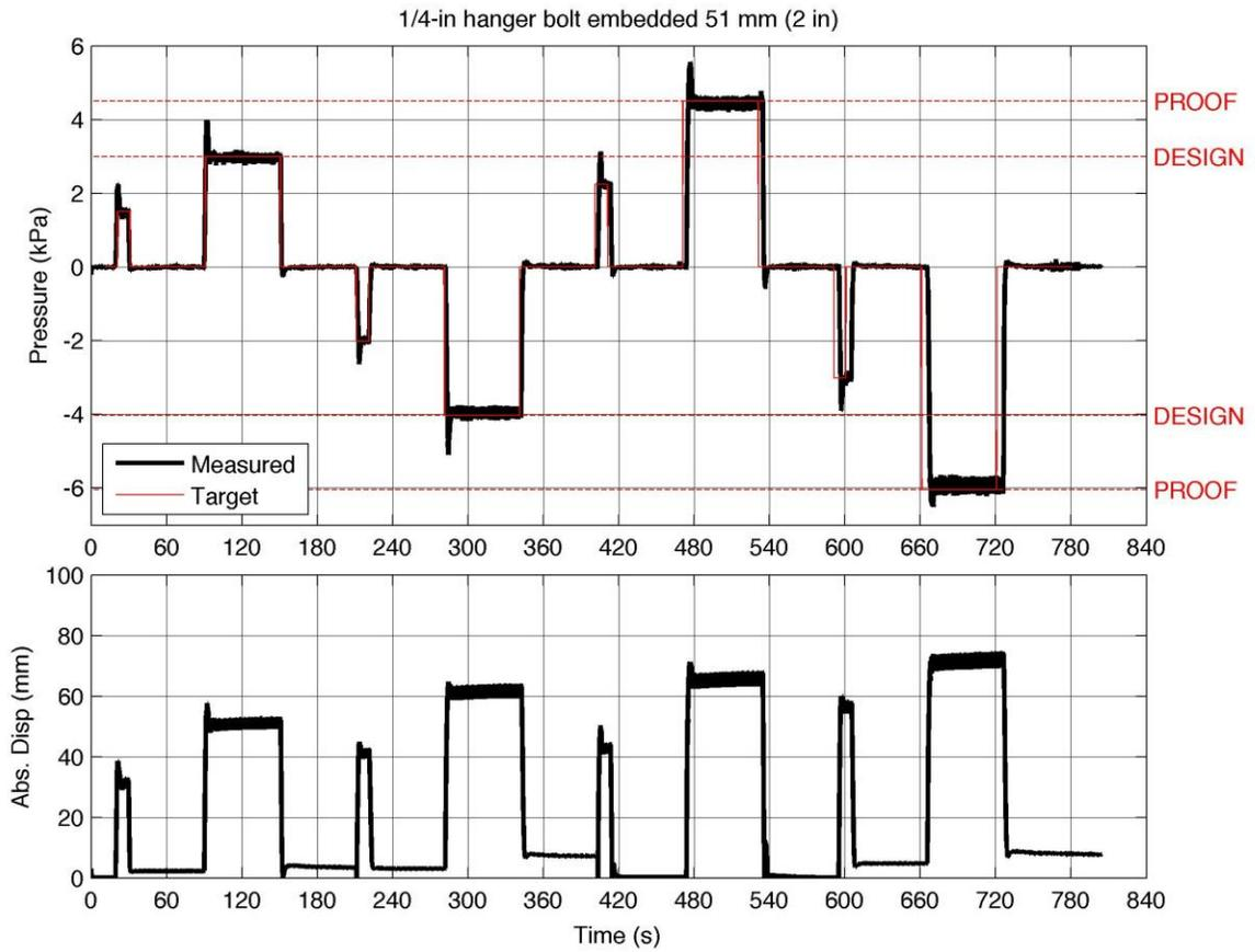
Figure 13. Static pressure loading sequence derived from ASTM E 330 for Case 1 (2.00 inch embedment)
