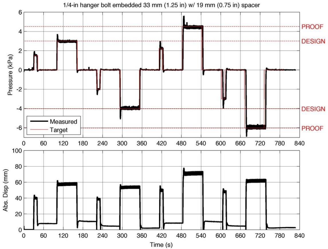
Figure 14. Static pressure loading sequence derived from ASTM E 330 for Case 2 (1.25 inch embedment)
