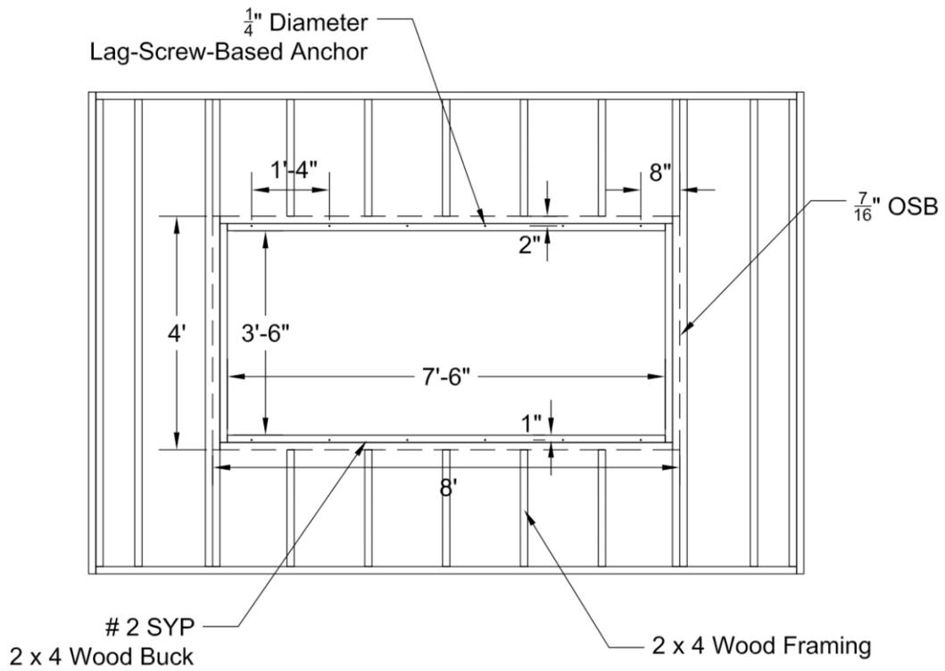
Figure 11. Wood frame wall configuration
