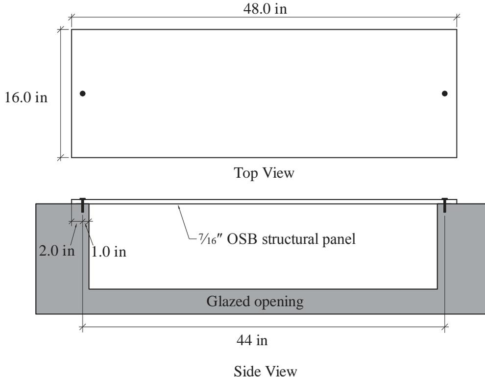
Figure 1. Panel used in experimental testing
