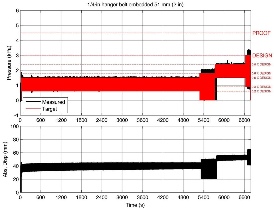
Figure 15. Cyclic pressure loading sequence derived from ASTM E1996 for Case 1 (2.00 inch embedment) for the positive pressure case
