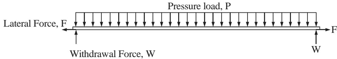
Figure 2. Free body diagram of panel undergoing beam action with catenary effects.
