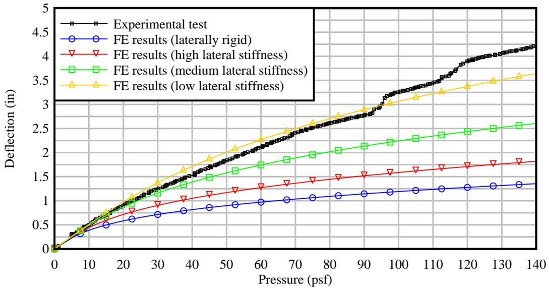
Figure 3. Comparison between experimentally-measured deflections and FEA results in the towards-the-building load direction
