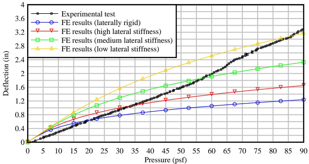
Figure 4. Comparison between experimentally-measured deflections and FEA results in the away-from-the-building load direction
