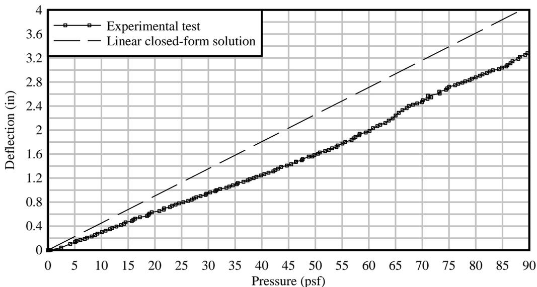
Figure 8. Validation of recommended closed form solution for deflection (load applied away from building)
