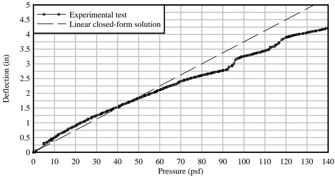
Figure 7. Validation of recommended closed form solution for deflection (load applied toward building)
