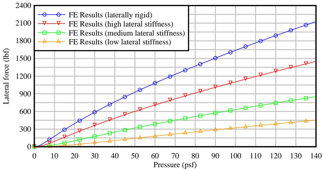
Figure 6. Comparison between FE lateral force results for different lateral stiffnesses in the away-from-the-building load direction
