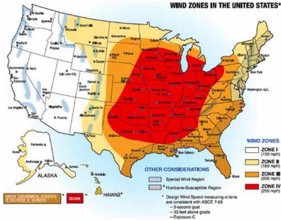
Figure 15: Wind zones from FEMA 320 based on ASCE 7-05 criteria. These same zones are also used in FEMA 361 and ICC 500 (Source: FEMA 320)
