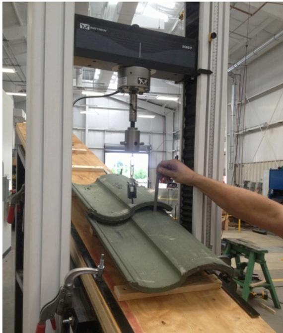
Figure 18. Mechanical uplift testing apparatus and testing arrangement
