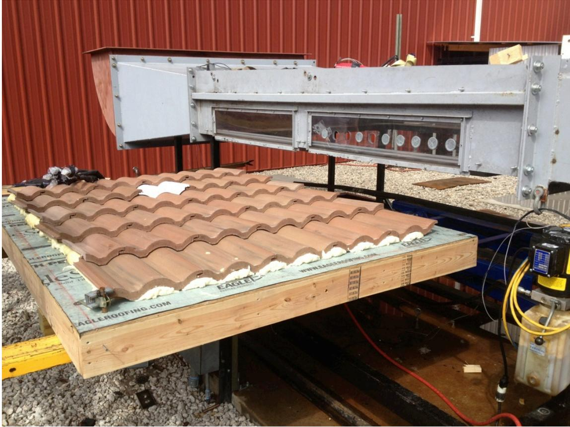
Figure 6. Foam adhesive set medium profile array studied in Phase II testing
