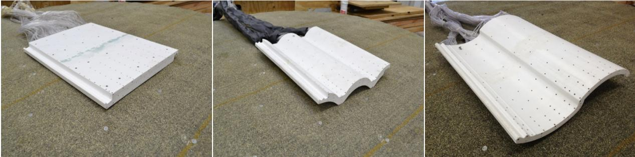
Figure 2. View of low-, medium- and high-profile model roofing tiles (shown left to right)
