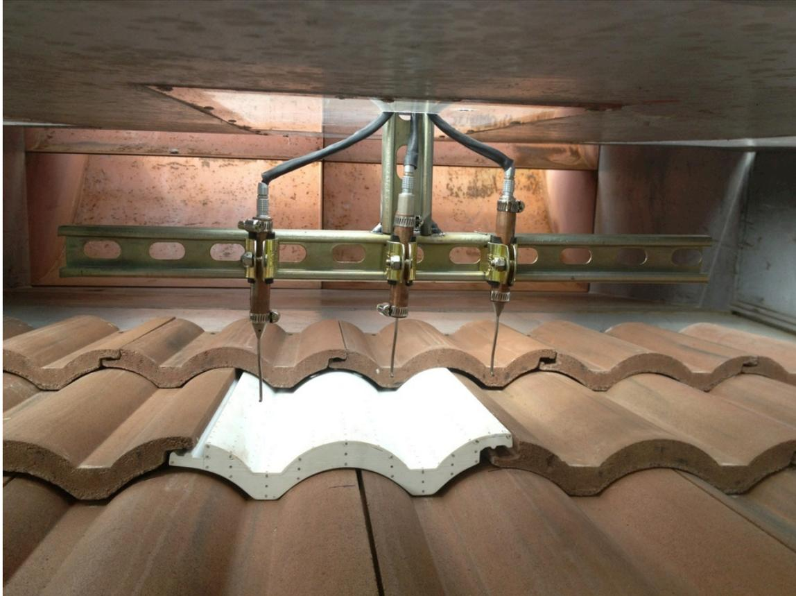
Figure 8. Cobra probe rake positioned above the medium profile roofing tile array
