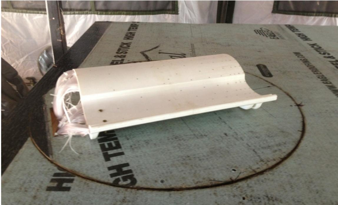
Figure 5. Mechanically fastened high profile model in Phase I configuration (45° wind angle)
