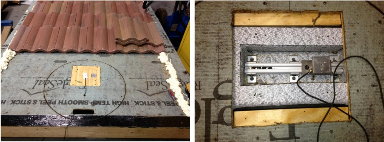
Figure 14. Medium profile load cell arrangement
