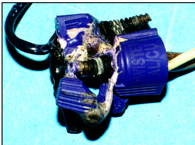
PLASTIC SHELLS SHELL MELTED AND CHARRED. THE CHARRING INDICATES THAT
