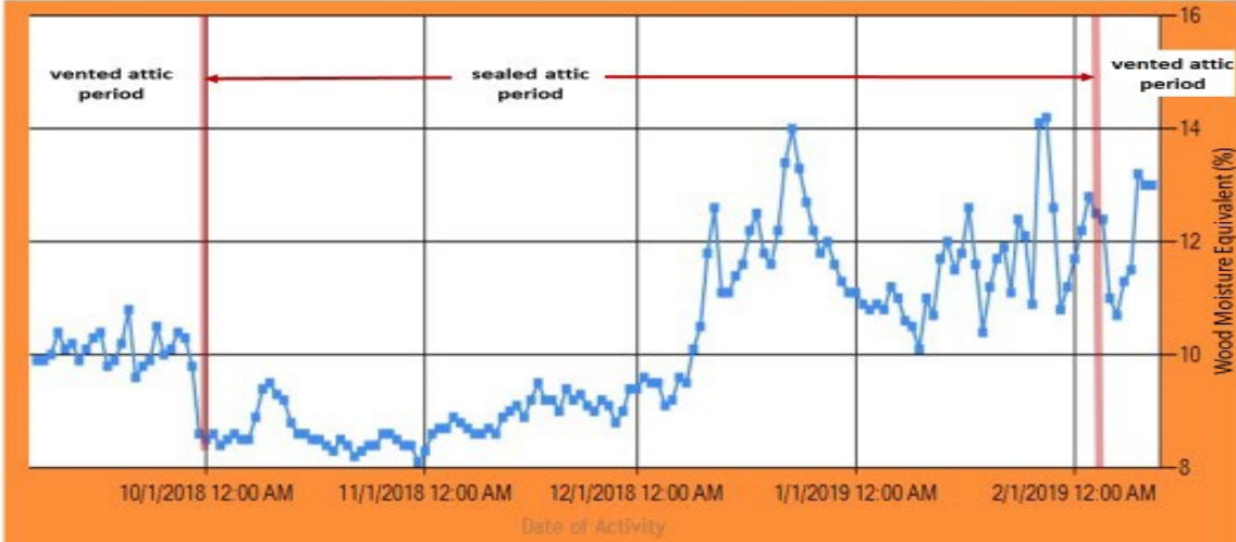
Figure 14. Wood Moisture Equivalent (WME) % at roof deck shows higher moisture during colder weather.
