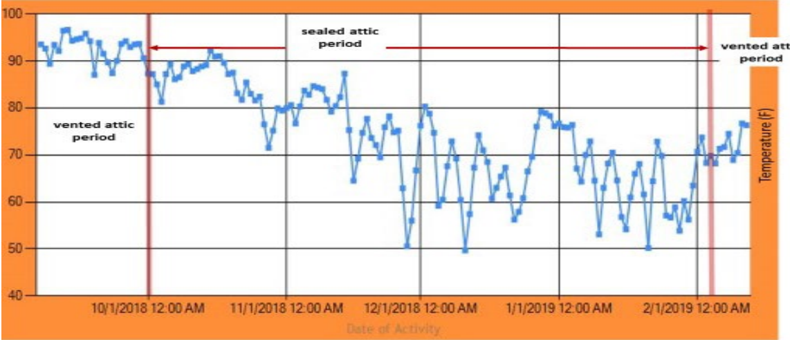
Figure 16. Colder attic deck temperatures trends coincide with higher WME % in Figure 14.
