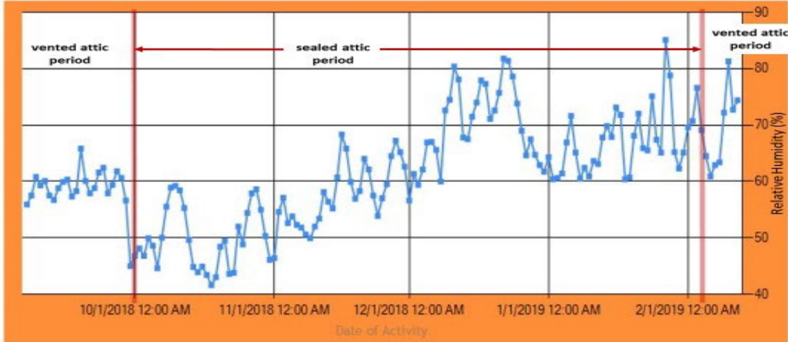
Figure 15. An increase in RH % at roof deck trends shows an expected direct relationship to WME% in Figure 14.
