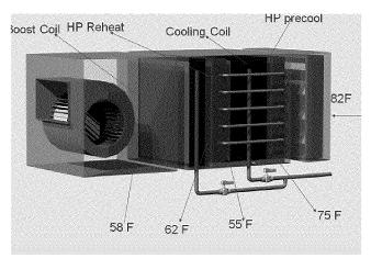
An example of the energy savings of a wrap-around heat pipe is shown on the below psychometric chart. The enthalpy savings (Btu per Pound of Dry Air) is represented below and shown as both Precool and Reheat.
