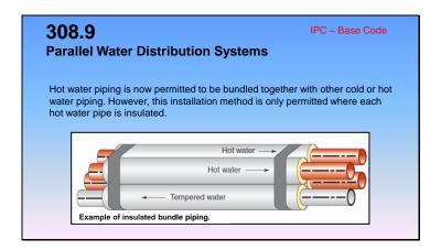
**308.9 Parallel Water Distribution Systems.** Piping bundles for manifold systems shall be supported in accordance with Table 308.5. Support at changes in direction shall be in accordance with the manufacturer's installation instructions. Where Hhot and cold water piping shall not be grouped in the same is bundled with cold or hot water piping, each hot water pipe shall be insulated.
