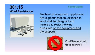
**301.15 Wind resistance.** Mechanical equipment, appliances and supports that are exposed to wind shall be designed and installed to resist the wind pressures on the equipment and the supports as determined in accordance with the *Florida Building Code, Building*. Roof-mounted mechanical units and supports shall be secured to the structure. The use of wood "sleepers" shall not be permitted.
