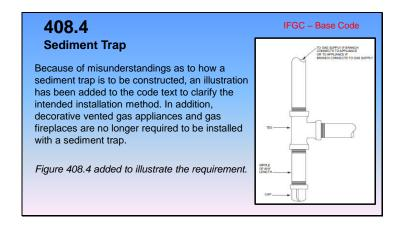
**408.4 Sediment Trap.** Where a sediment trap is not incorporated as part of the appliance, a sediment trap shall be installed
