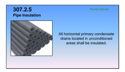
**307.2.5 Pipe insulation.** All horizontal primary condensate drains within unconditioned areas shall be insulated to prevent condensation from forming on the exterior of the drain pipe.
