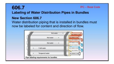
606.7 Labeling of Water Distribution Pipes in Bundles. Where water distribution piping is bundled at installation, each pipe in the bundle shall be identified using stenciling or commercially available pipe labels. The identification shall indicate the pipe contents and the direction of flow in the pipe. The interval of the identification markings on the pipe shall not exceed 25 feet. There shall be not less than one identification label on each pipe in each room, space, or story.
