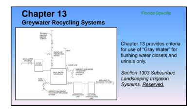
**1301.1 Scope.** The provisions of Chapter 13 shall govern the materials, design, construction and installation of gray water systems for flushing of water closets and urinals and for subsurface landscape irrigation. See Figures 1301.1(1) and 1301.1(2).
