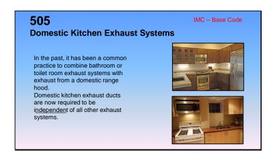
**505.1 Domestic Systems.** Where domestic range hoods and domestic appliances equipped with downdraft exhaust are located within dwelling units, such hoods and appliances shall discharge to he outdoors through sheet metal ducts constructed of galvanized steel, stainless steel, aluminum or copper. Such ducts shall have smooth inner walls, and shall be air tight, and shall be equipped with a back-draft damper, and shall be independent of all other exhaust systems. **Exceptions:**
