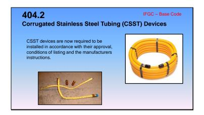
**404.2 CSST.** CSST piping systems shall be installed in accordance with the terms of their approval, the conditions of listing, the manufacturer's installation instructions and this code.
