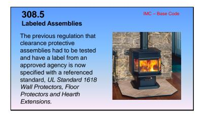
**308.5 Labeled Assemblies:** The allowable clearance reduction shall be based on an approved reduced clearance protective
