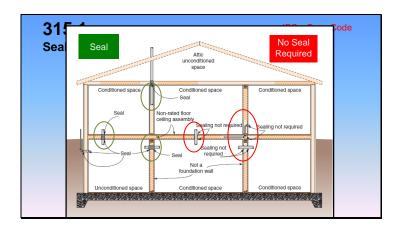
**305.4** <u>315.1</u> <u>Sleeves Sealing of Annular Spaces.</u> The annular spaces between the outside of a pipe and the inside of a pipe sleeves, and pipes or between the outside of a pipe and an opening in a building envelope wall, floor, or ceiling assembly penetrated by a pipe shall be filled or tightly caulked sealed in an approved manner with caulking material or closed with a gasketing system. The caulking
