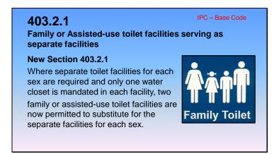
403.2.1 Family or Assisted-Use Toilet Facilities Serving as Separate Facilities. Where a building or tenant space requires a separate toilet facility for each sex and each toilet facility is required to have only one water closet, two family/assisted-use toilet facilities shall be permitted to serve as the required separate facilities. Family or assisted use toilet facilities shall not be required to be identified for exclusive use by either sex as required by Section 403.4.
