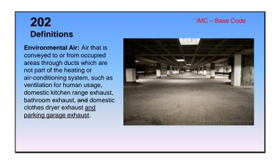
**202 Environmental Air:** Air that is conveyed to or from occupied areas through ducts which are not part of the heating or air-conditioning system, such as ventilation for human usage, domestic kitchen range exhaust, bathroom exhaust, and domestic clothes dryer exhaust and parking garage exhaust.
