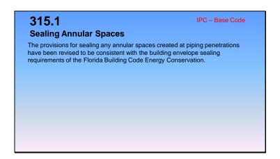
**305.4** 315.1 Sleeves Sealing of Annular Spaces. The annular spaces between the outside of a pipe and the inside of a pipe sleeves, and pipes or between the outside of a pipe and an opening in a building envelope wall, floor, or ceiling assembly penetrated by a pipe shall be filled or tightly caulked sealed in an approved manner with caulking material or closed with a gasketing system. The caulking
