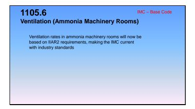
**1105.6 Ventilation.** Machinery rooms shall be mechanically ventilated to the outdoors. Mechanical ventilation shall be capable of exhausting the minimum quality of air both at the normal operating and emergency conditions. Multiple fans or multispeed fans shall be allowed
