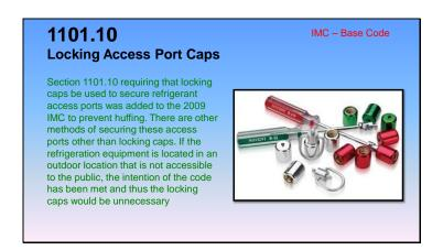
**1101.10 Locking Access Port Caps.** Refrigerant circuit access ports located outdoors shall be fitted with locking-type tamper-resistant caps <u>or shall be otherwise secured to prevent</u> unauthorized access.
