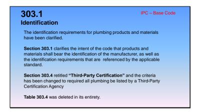
**303.1 Identification.** Each length of pipe and each pipe fitting, trap, fixture, material, and device utilized in a plumbing system shall bear the identification of the manufacturer <u>and any markings</u> required by the applicable referenced standards.
