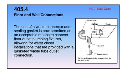
**405.4 Floor and Wall Drainage Connections.** Connections between the drain and floor outlet plumbing fixtures shall be made
