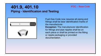
**401.9 Identification.** Each length of pipe and tubing and each pipe fitting, utilized in a fuel gas system, shall bear the identification of the manufacturer.
