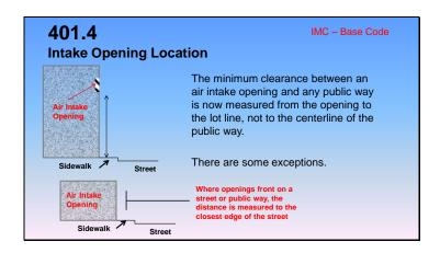
**401.4 Intake Opening Location.** Air intake openings shall comply with all of the following: **1.** Intake openings shall be located a minimum of 10 feet (3048 mm) from lot lines or buildings on the same lot. Where openings front on a street or public way, the distance shall be measured to the centerline of the street or public way.
