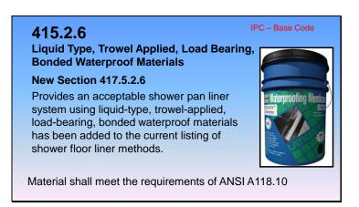
417.5.2.6 Liquid Type, Trowel Applied, Load Bearing, Bonded Waterproof Materials. Liquid type, trowel applied load bearing, bonded waterproof materials shall meet the requirements of ANSI A118.10 and shall be applied in accordance with the manufacturer's installation instructions.
