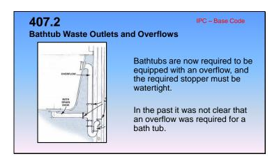
**407.2 Bathtub Waste Outlets** <u>and Overflows</u>. Bathtubs shall <u>have</u> <u>be equipped with a</u> waste outlets and an overflow outlet. <u>The minimum outlets shall of be connected to waste tubing or piping not less than 1 ½ inches (38 mm) in diameter., and the waste outlet shall be equipped with an approved <u>watertight</u> stopper.</u>
