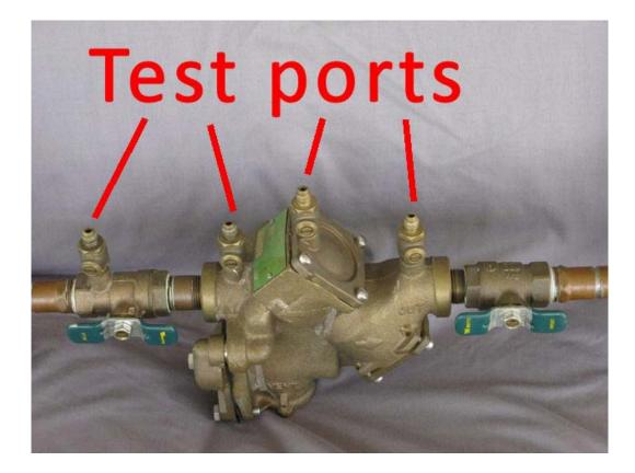
RP and DC valves are complicated and prone to failure. Because of this they must be tested every year or two just to be sure they're even working. This testing is done by way of the four test ports that are located across the top of both RP and DC valves.
