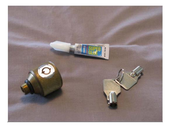
So, the valve manufacturers came up with Test Port Locks that are purported to prevent access to the potable water. The concept was that the outer shell could be unlocked from the center part and a terrorist could not then unscrew the lock to gain access to the water supply through the ports.
