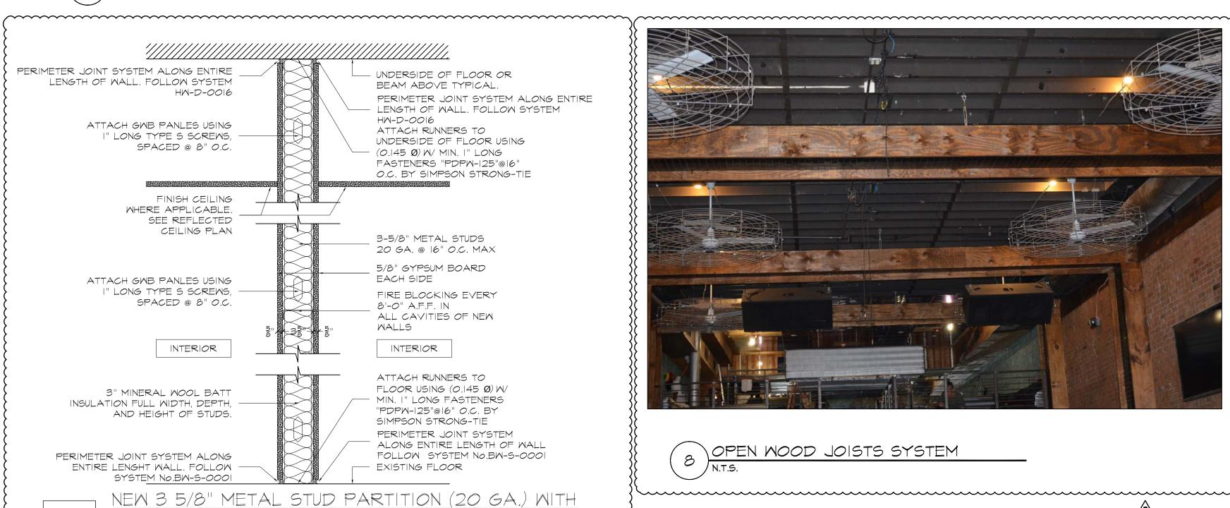
NEW 3 5/8" METAL STUD PARTITION (20 GA.) WITH ONE LAYER OF 5/8" GYPSUM BOARD ON EACH SIDE ÚL DESIGN No. U419) "I HOUR RATED-51 STC MIN. SCALE: | |/2" = |'-0"
