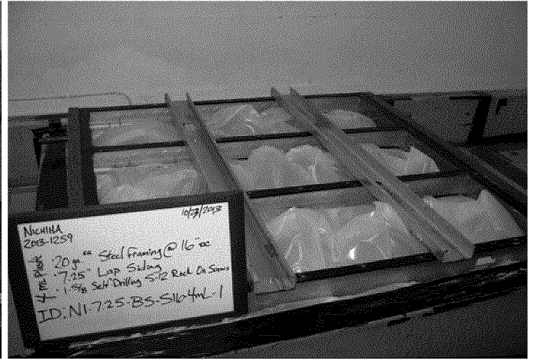
Typical Test Setup (with bracing)
