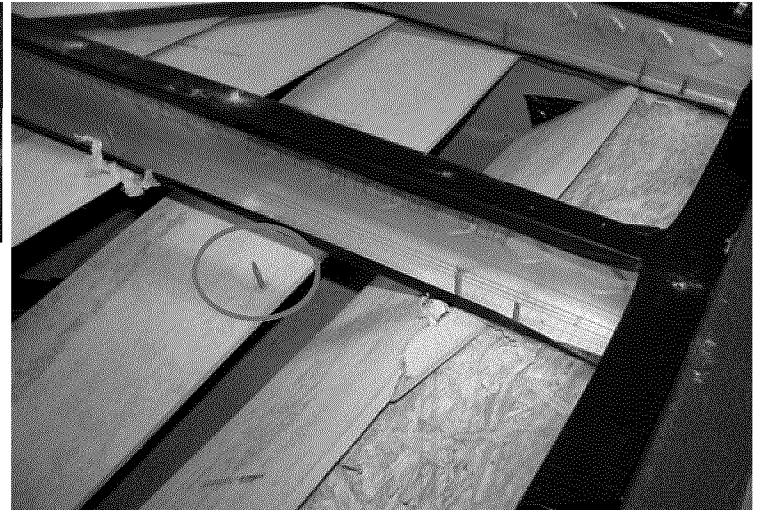
CT-7.25-BS-S16-2mT-1 Failure (fastener withdrawal)
