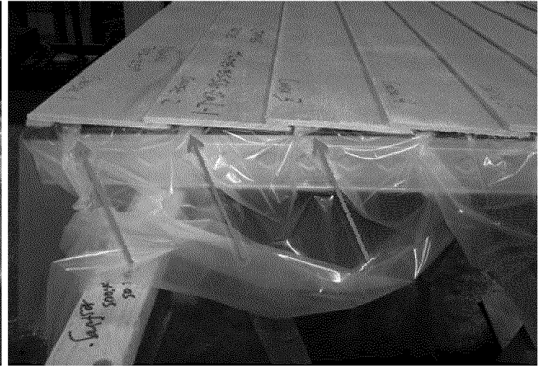
Typical folds at each siding course - Loose Film
